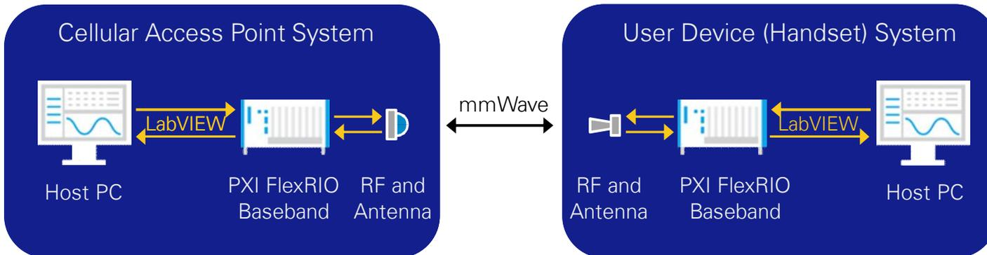
The experimental 5G PoC system will be implemented using National Instruments' baseband modules which make up the state-of-the-art system for rapid prototyping of 5G air interfaces today.
