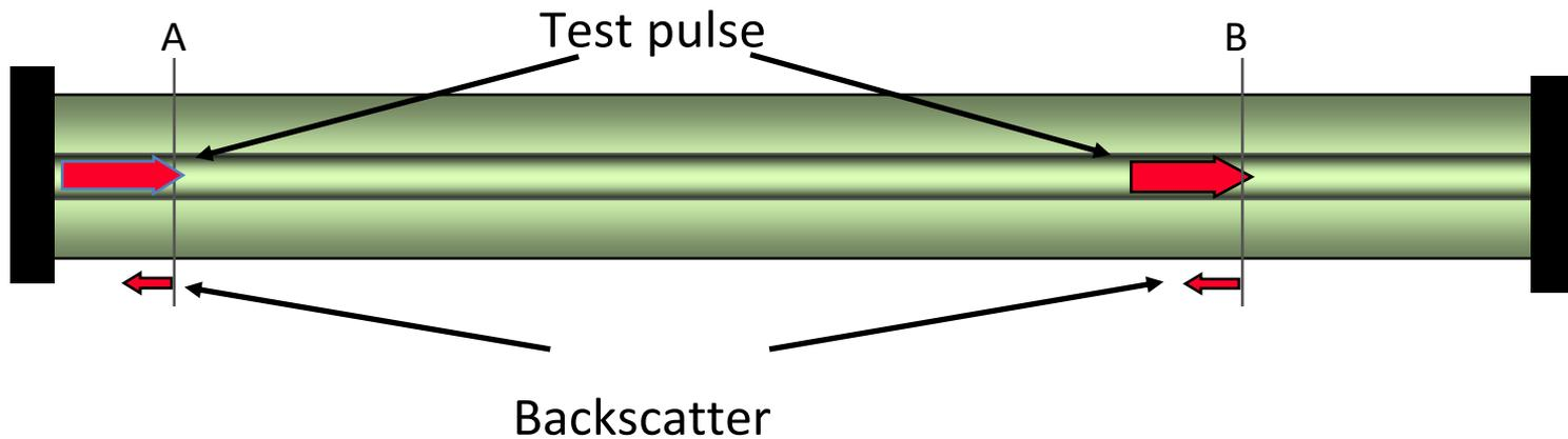
Backscatter is directly related to the level of light in the test pulse. As the level of light in the pulse width decreases with distance, so does the backscatter it produces.
