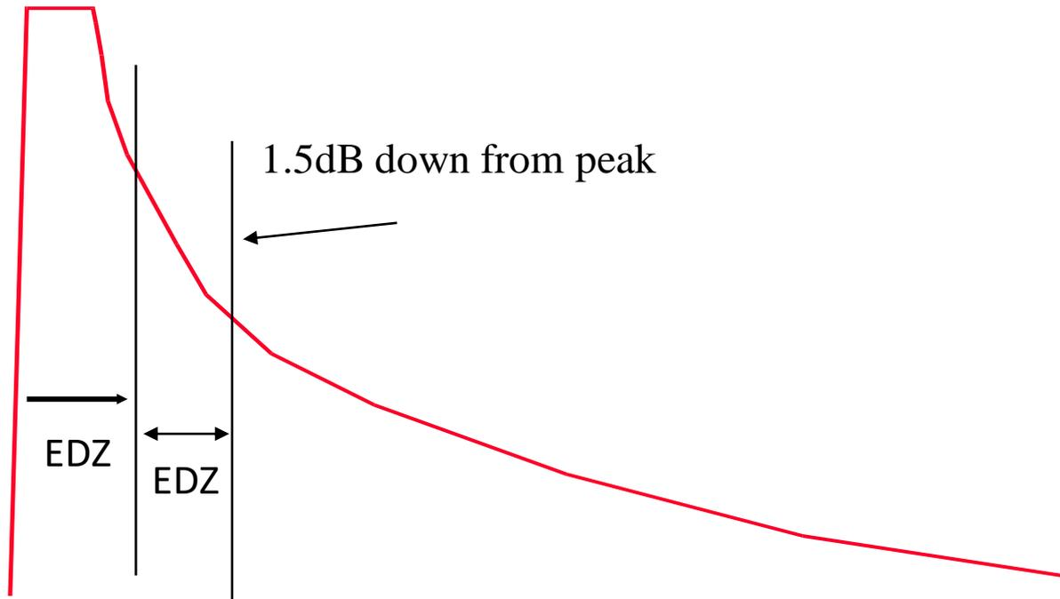
**An OTDR's Initial Event Deadzone will have this appearance without a fiber connected to the OTDR.**
