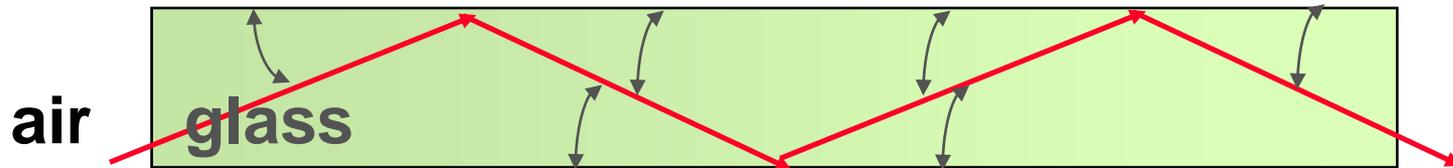
As long as the light ray stays at the Critical Angle or less as it hits the air-glass interface, it will remain in the fiber until it reaches the other end.
