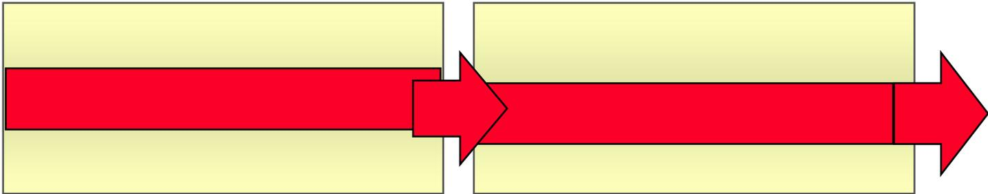
Off-center core in second fiber does not receive all the light from the first fiber. The amount of light lost is the Splice Loss.
