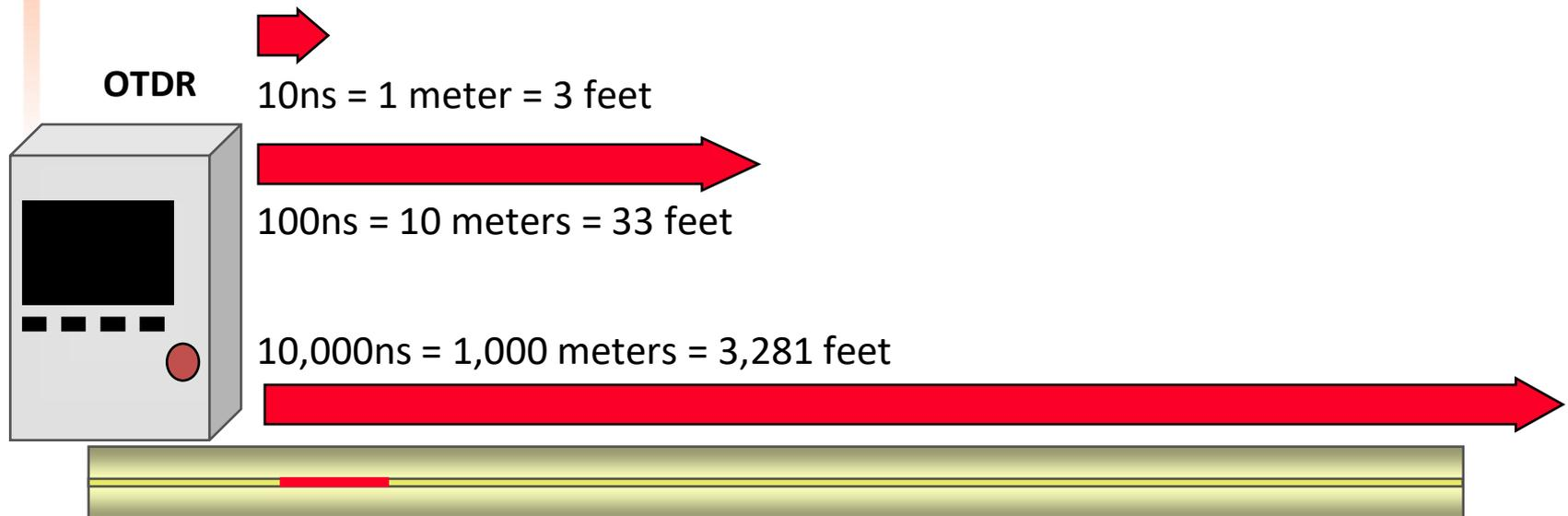
*Only one test pulse is allowed in the fiber at any time.*
