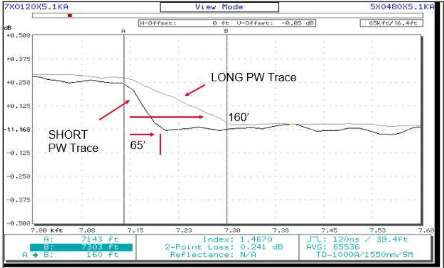
Long Pulse Width takes longer to make the transition from backscatter of first fiber to backscatter of second fiber. Short Pulse Width makes a sharper transition.
