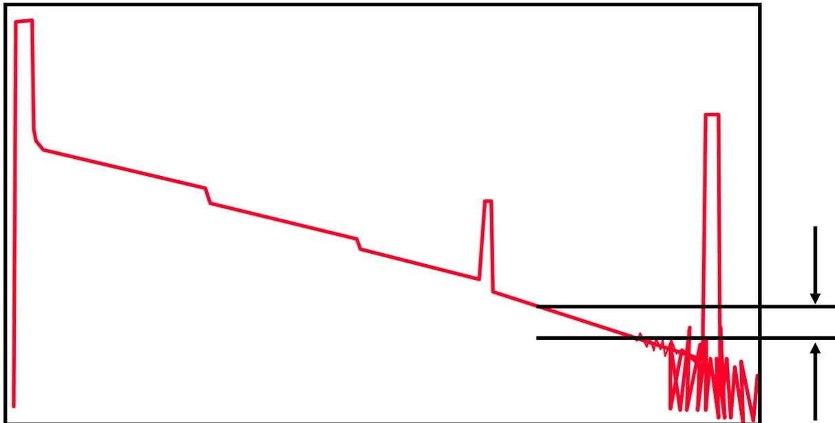
FAS needs 3dB between backscatter and noise level to find fiber end, or else gives “Out of Range” warning.
