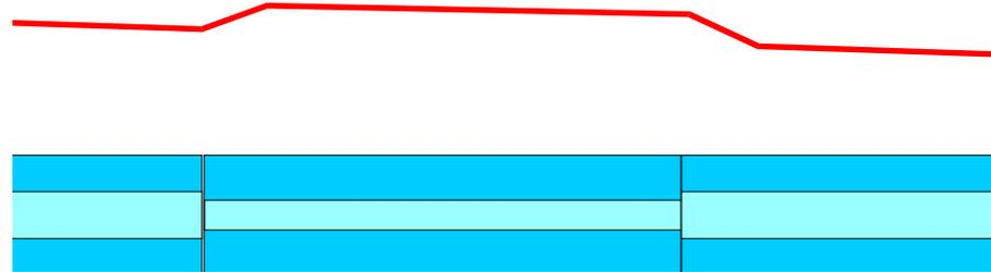
$$\text{Total Backscatter} = -10 \log \left( \frac{W1}{W2} \right)^2 \text{ dB}$$
