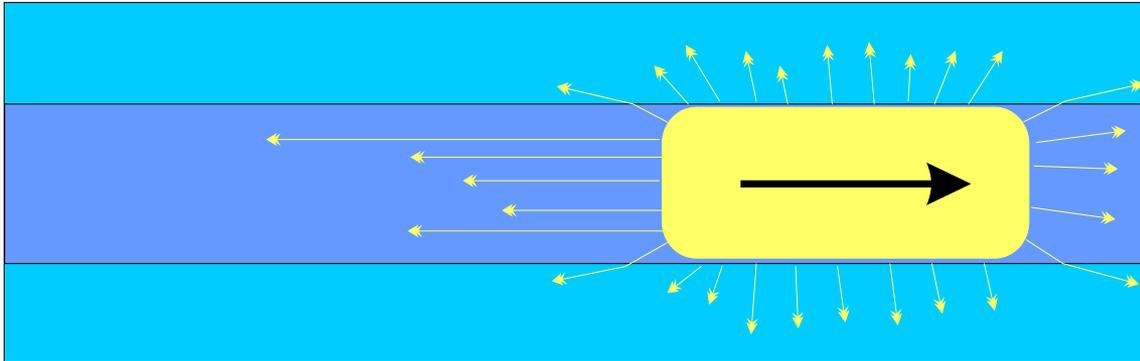
**Rayleigh scattering is the primary cause of light loss as the pulse of light travels down the fiber.**
