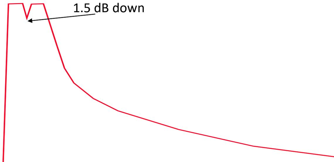
However, should the OTDR display the trace above when connected to a fiber at the patch panel, it can easily be seen that there are two events. The first is at the OTDR, the second is where the fiber is broken.
