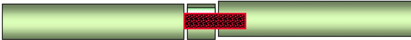
Long PW produces longer DZ, preventing the detection & measurement of individual splices. The PW strikes the second connection before clearing the first connection.
