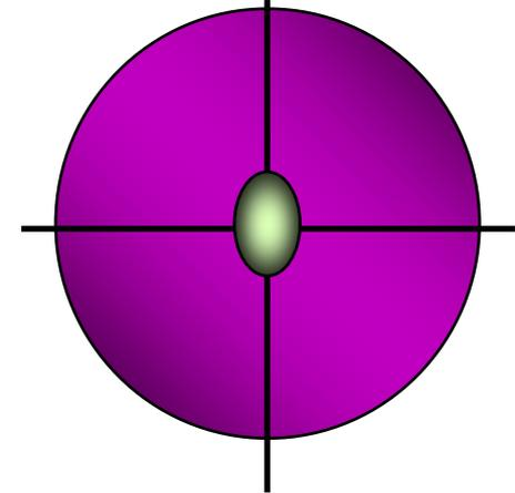
All fibers are allowed a certain tolerance in the core/cladding geometry. This can cause light loss at joints between fibers.
