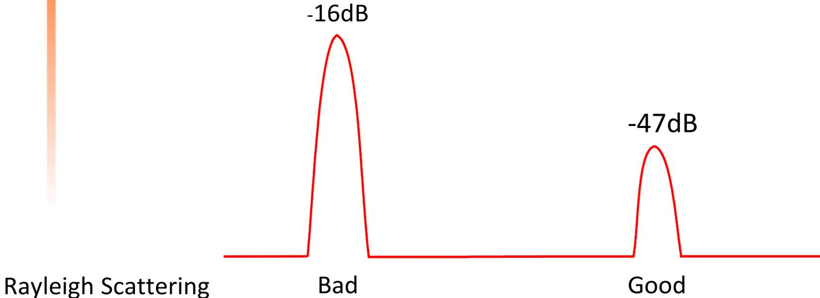
**Reflections are measured from the receiver's point of view. Reflected light is power lost to the receiver and is therefore a negative number.**
