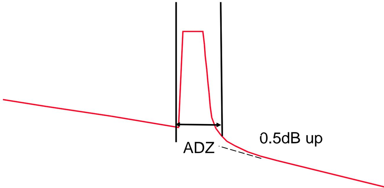
The distance of the Attenuation Deadzone is from the start of a reflective event until 0.5dB up from the backscatter level after the reflection.
