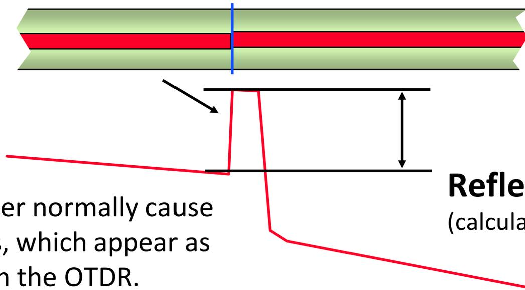
Ends of fiber normally cause reflections, which appear as “spikes” on the OTDR.
