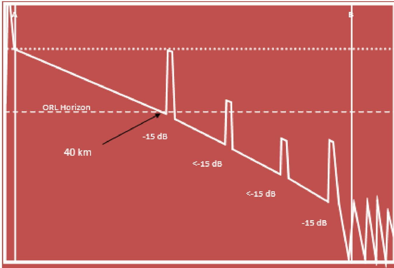
Reflections returning from farther than 40km will have not effect on the stability of the transmitter. Accurate ORL measurements do not require measuring to the end of a 150 km link. Only the first 40 km matter.
