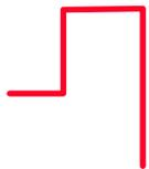
Cable End = point in fiber where signal level drops off. Means “Out of Range” or “Out of Distance”.
