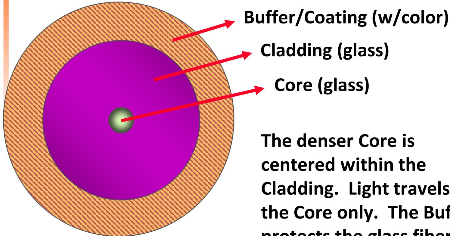
The denser Core is centered within the Cladding. Light travels in the Core only. The Buffer protects the glass fiber.
