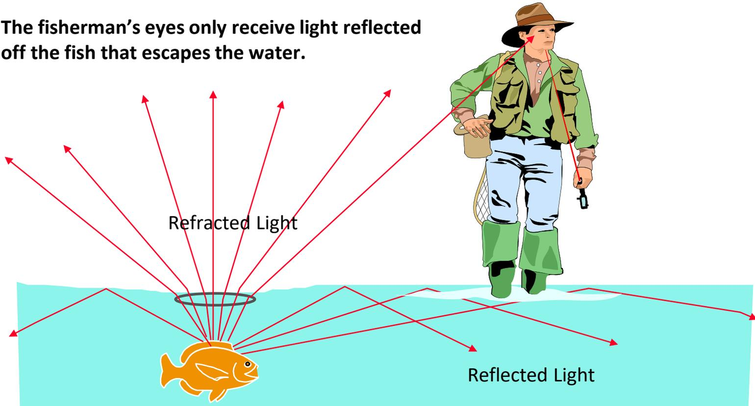
Light rays reflecting off the fish that strike the surface of the water at an angle outside that defined by the circle do not escape but are reflected back into the water.
